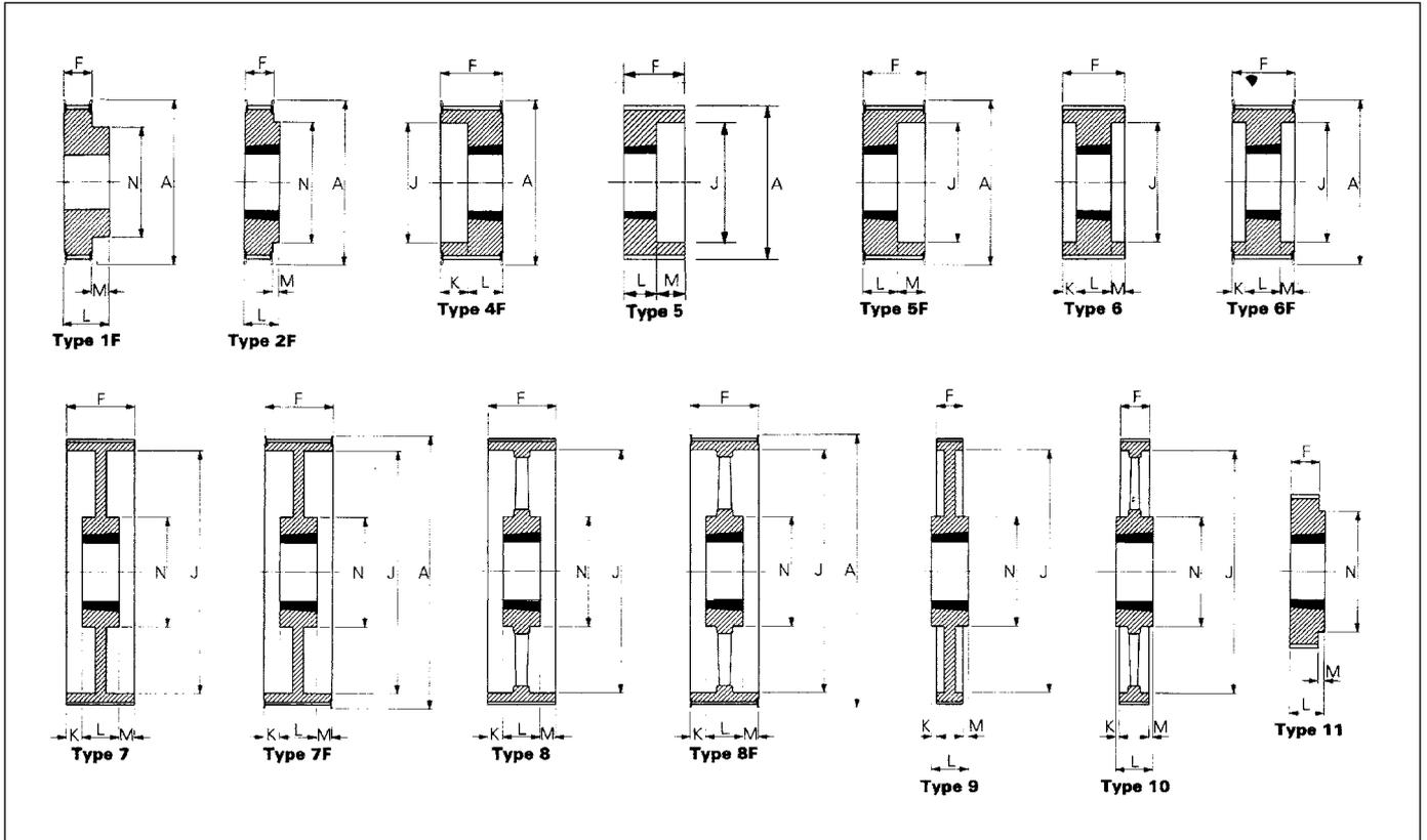
**5mm PITCH (5M) HTD PULLEYS (FOR USE WITH HTD BELTS ONLY)**
